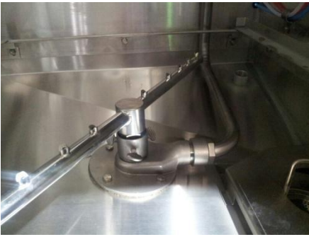
Spray arm, base w/thumb screws
