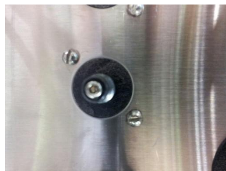
Chemical alarm barb adjusting screw *
