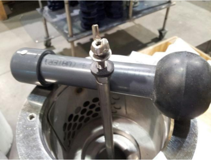
ET (gravity) drain ball, note rubber washer on push rod
