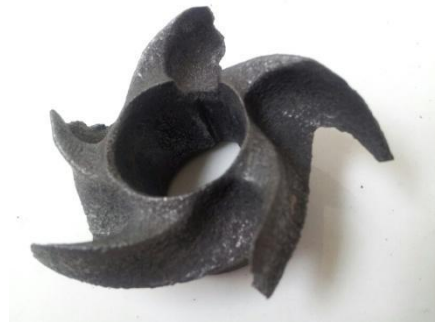
Impeller damaged from high acid solution
