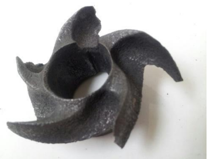
Impeller damaged from high acid solution
