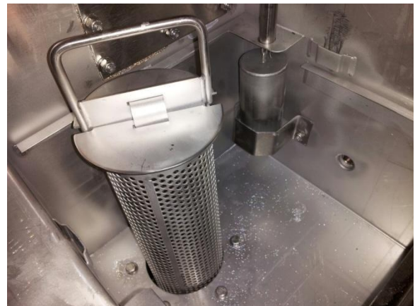
Pump filter in drain sump
