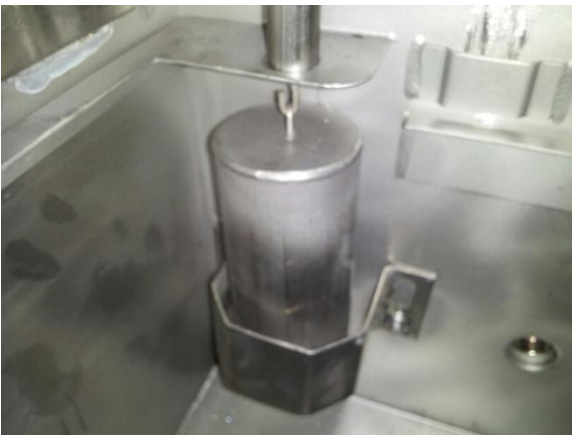
Wash tank float and tank overflow
