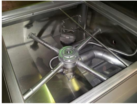
Wash arm w/bearing installed on base
