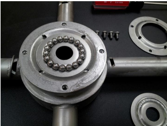
Top race removed, ball bearings for replacement
