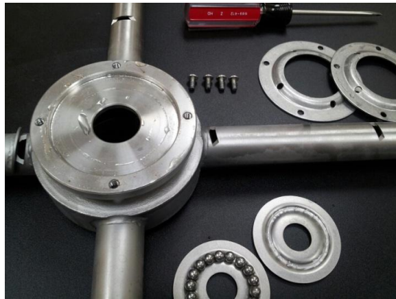
Races are interchangeable, capture shells are also
