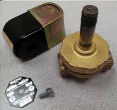
Remove screw and coil from tube
