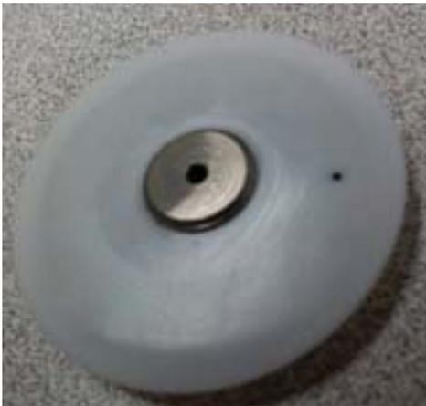
Turn over the diaphragm inspect near the rivet head
