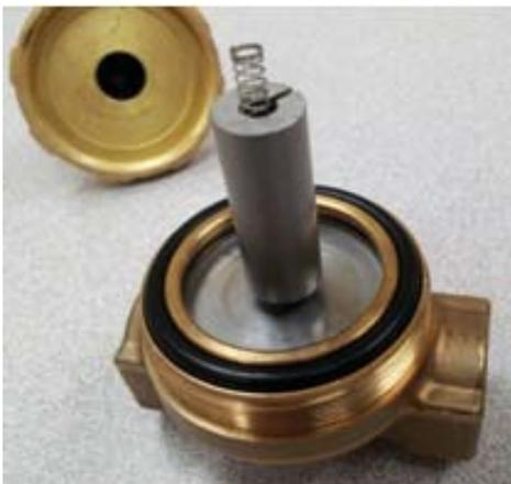
Correct plunger placement, spring on top
