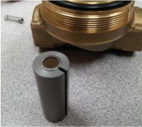
Inspect the gasket in bottom of the plunger
