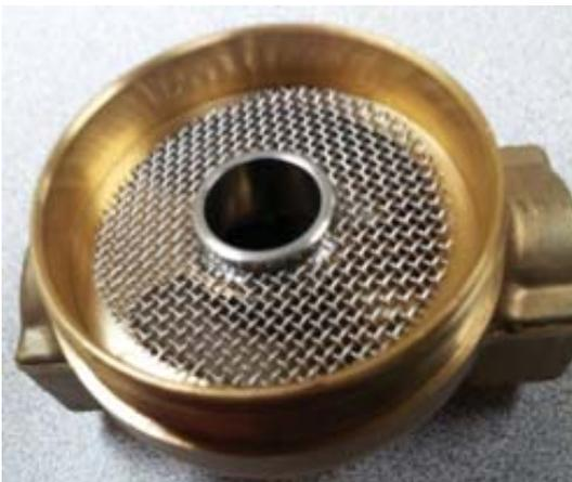
Remove the o-ring retainer, remove the screen
