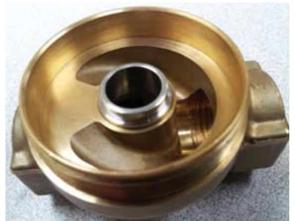
Remove any material or debris from the body. Inspect the center ring for cuts or damage to the surface. If the stainless seat (center ring ) is rough or cut, the valve body must be replaced.
