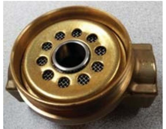
A cut or indent would stop sealing on the center ring
