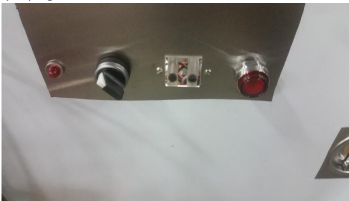
Cycle light, master switch, chemical sight window, red start switch
