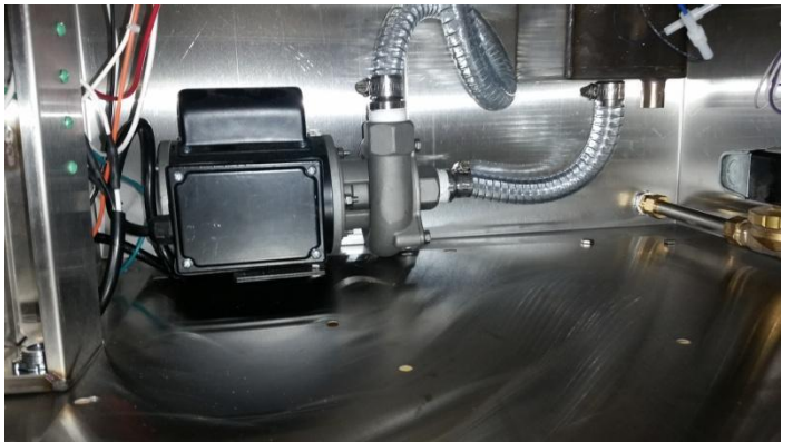
Wash pump with rinse pump removed
