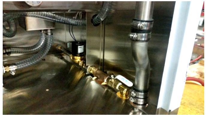
Showing 1/2" H 2 O solenoid, also stainless 1.5" drain tube
