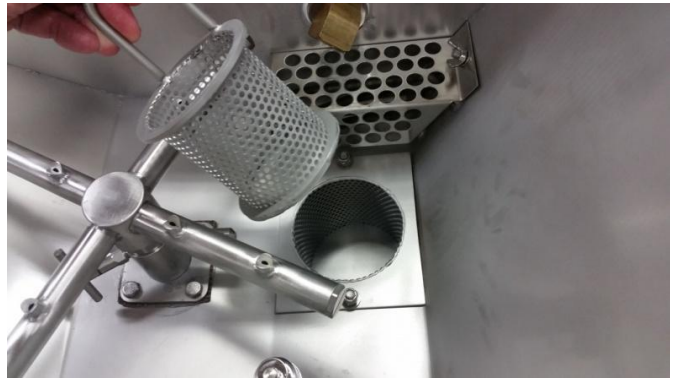
Showing pump scrap basket
