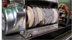
The arrow is pointed at the left-side wheel of the cam which is used to lengthen or shorten the low cam or the time ON for the respective switch. Adjustable cams are colored either black or gray
