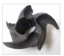
Impeller damaged from high acid solution
