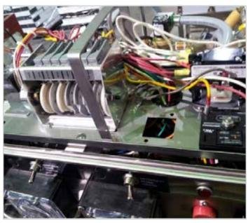
Showing control tray installed in normal position
