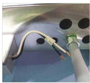
Showing power connection box for 120v wiring
