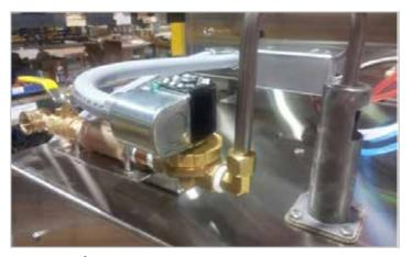
Showing 1/2" female pipe inlet, ball valve, y-line filter,water solenoid, ASSE approved air gap (backflow preventer)
