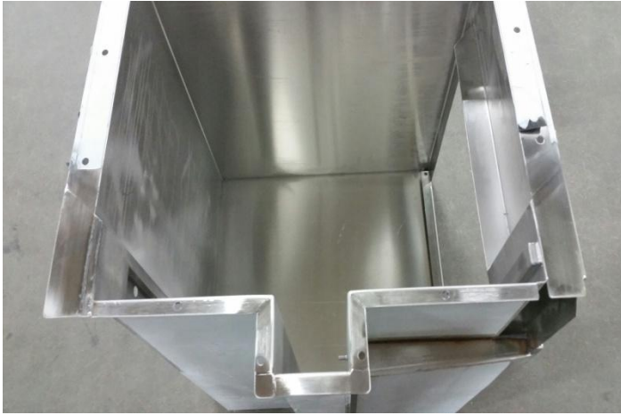
Lower pan of loader fits inside the DM tank and bolts
