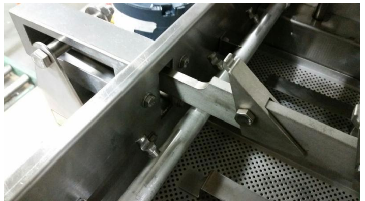
Conveyor bar attaches to rocker arm on clean side of DM
