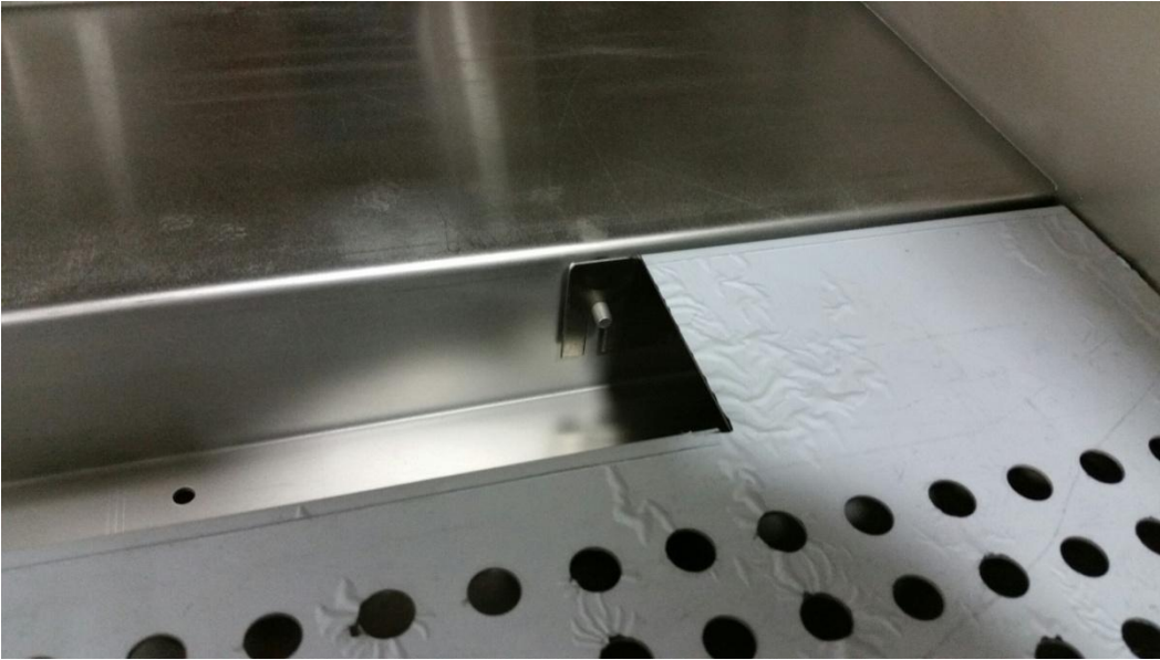
Ramp bolts in place for racks to slide over the conveyor bar.
