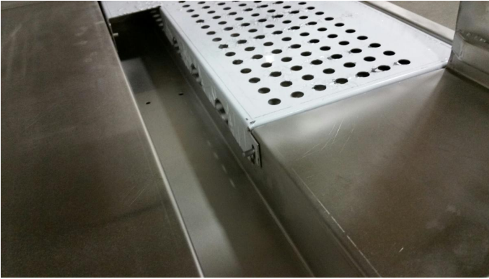
Ramp over the conveyor bar trough
