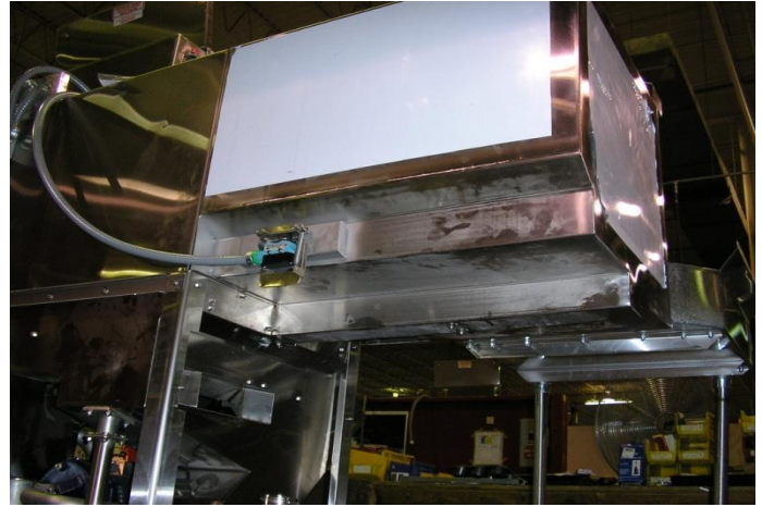
Showing start switch attached to the pocket
