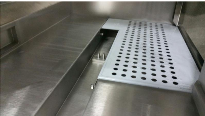
Ramp installed and held by two studs and lock nuts.
