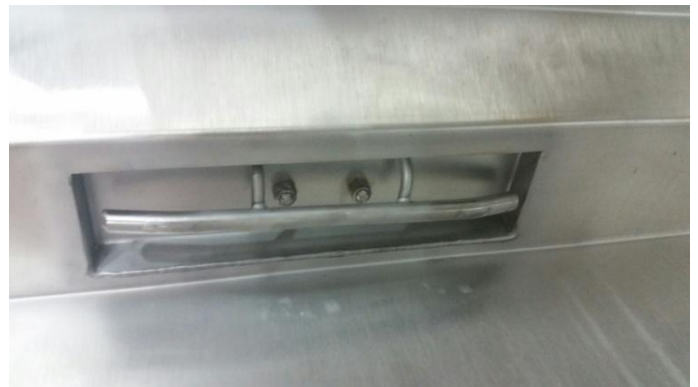
Bumper attached thru pocket to tilt plate
