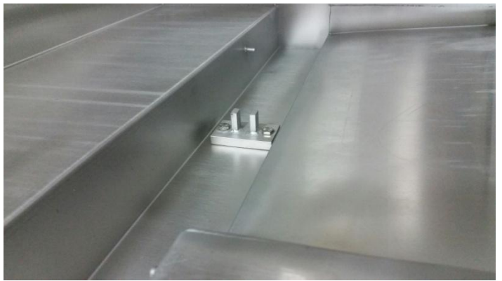
Rubbing block (285-6187) bolted in place
