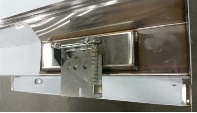
Showing tilt plate and holder for switch shuttle
