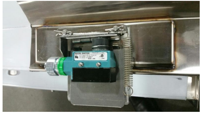
Switch bolted to shuttle and installed on tilt plate
