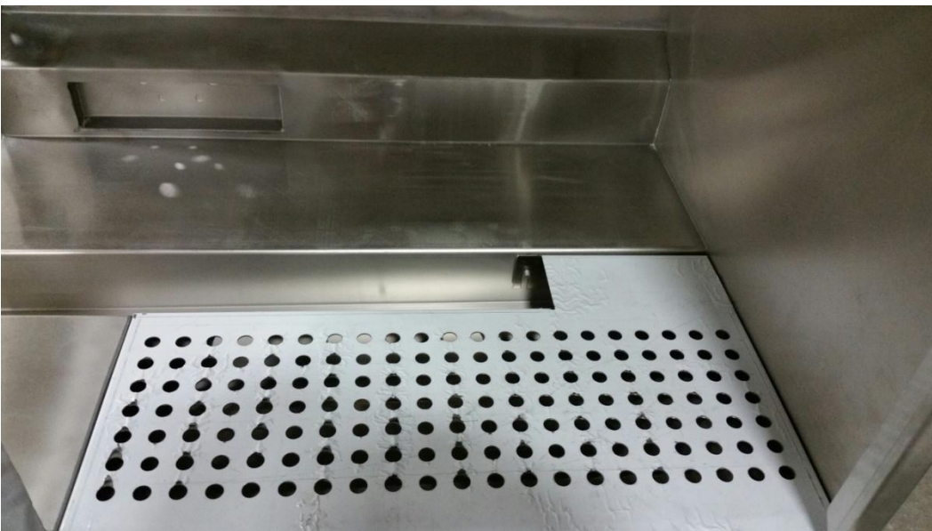
Showing the full ramp and the pocket for the start switch in upper left of picture
