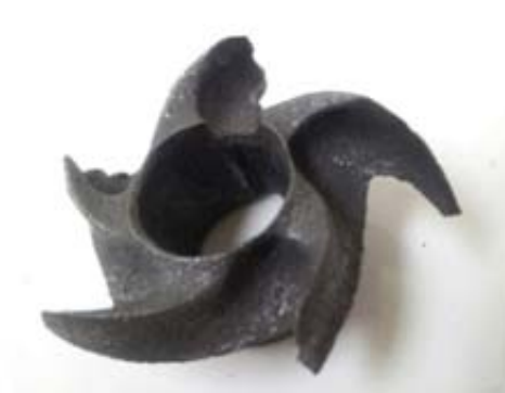
Impeller damaged from high acid solution
