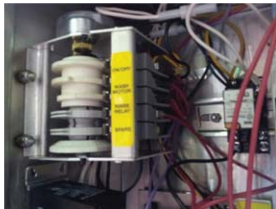
Cam timer with 3 fixed operational cams, 2 adjustable
