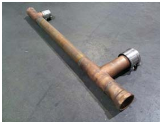
HT-25 drain manifold with "no-hub" connectors
