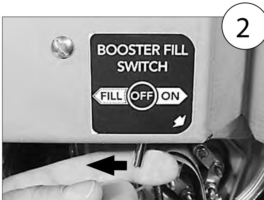
6. PUSH the booster fill switch to the ON position and release.
