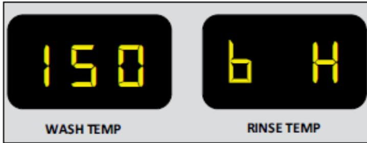
Booster overtemp lockout because booster temperature is greater than 210°F.
