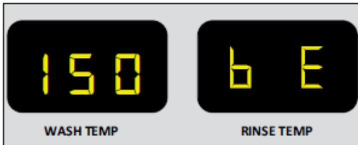
Booster thermistor is defective or disconnected, broken wires.
