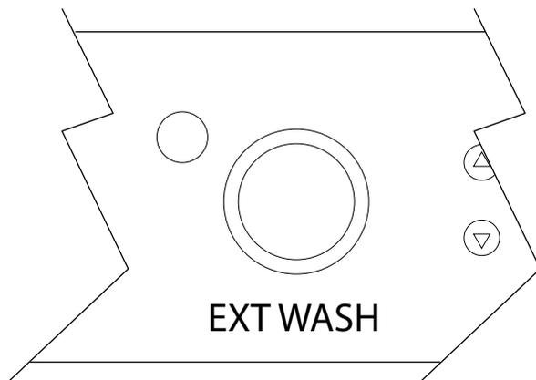
Press the EXT WASH button to place the machine into the extended wash mode to clean heavily soiled wares.
