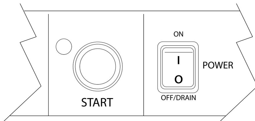
1. Push the illuminated power switch down to the OFF/DRAIN position. The power switch light will go out.
