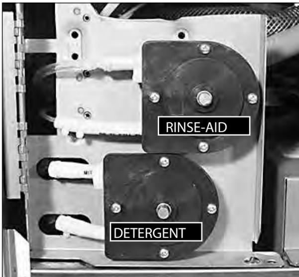
The pumps are located on the left-side behind the lower front panel of the dishwasher.
