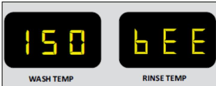
Both booster and final rinse display thermistors are defective, unplugged, or open or broken wires between the display and thermistor.
