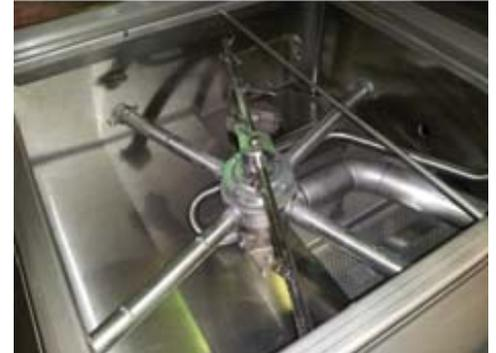
Final rinse arm twisted into transfer tube
