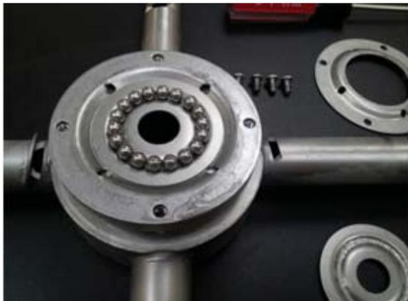
Top race removed, ball bearings for replacement
