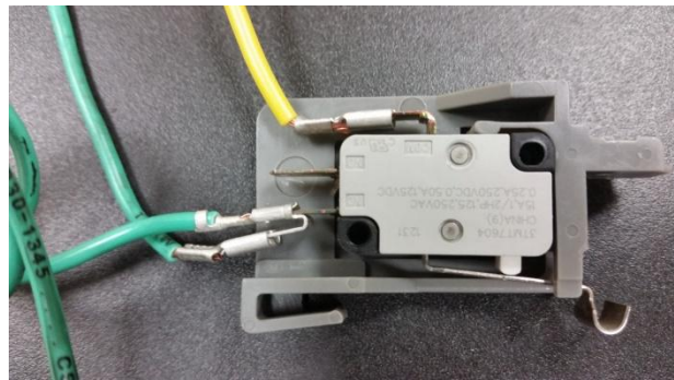
Wire connections to the cam timer sanitizer
