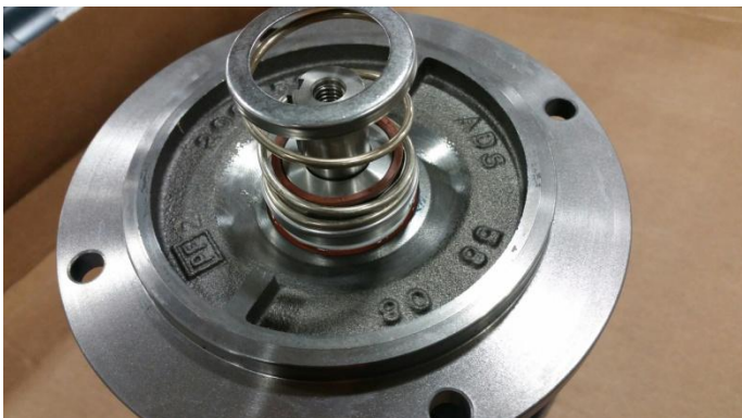
Using dish soap again, press graphite till it seats on ceramic
