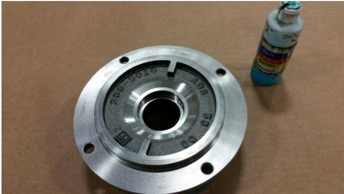
Lubricate the pump housing with some dish soap
