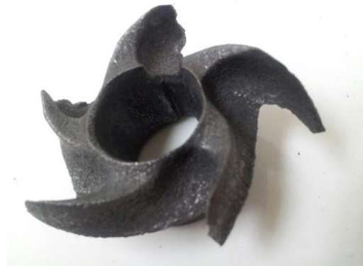
Result of spinning impeller in high ratio acid solution
