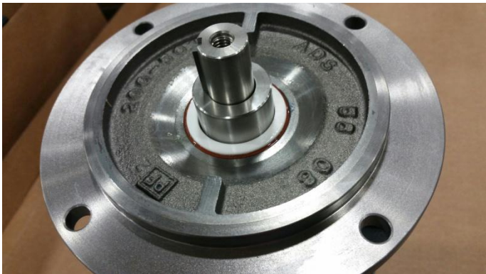
Press the ceramic half of the seal w/boot into the housing
