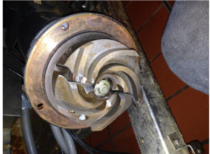
Results of key shifting in the shaft and motor
