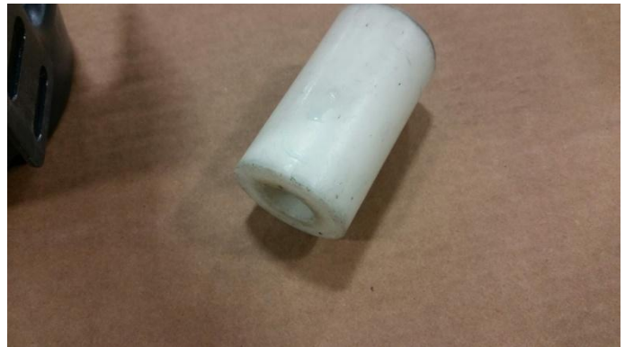
Use 1.5" OD plastic tube to press seal till firmly seated
