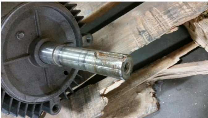
Showing key way damaged
