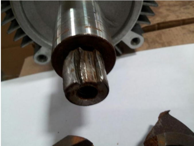
Motor with damaged key way
