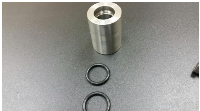
Motor shaft sleeve w/inner o-rings
