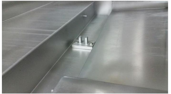
Rubbing block (285-6187) bolted in place
