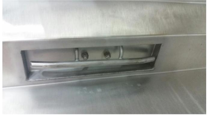
Bumper attached thru pocket to tilt plate
