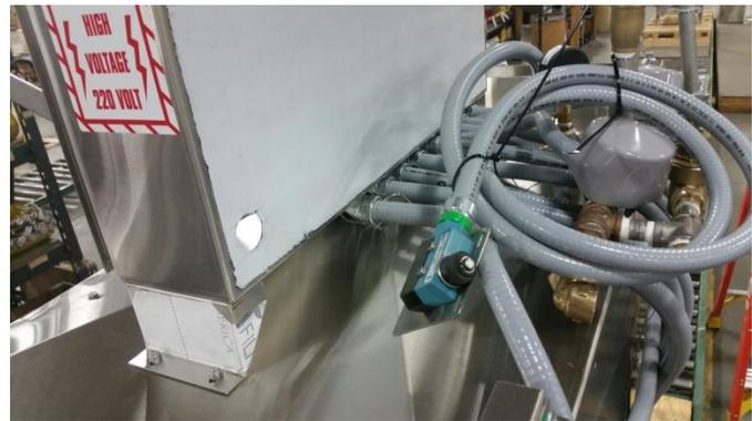
For shipping purposes, the connection to the start switch is removed, coiled and tied to the top of the machine.
