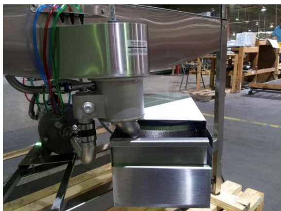
5CD right-front shown (box does bolt in place) Box, cover and tray assembly
