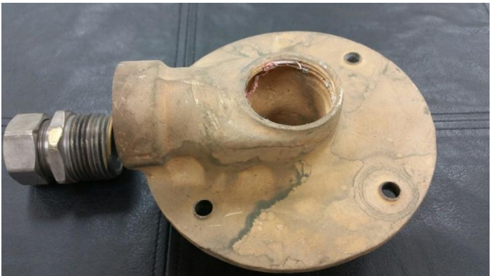
Chemicals erode the base, threads would no longer fit
