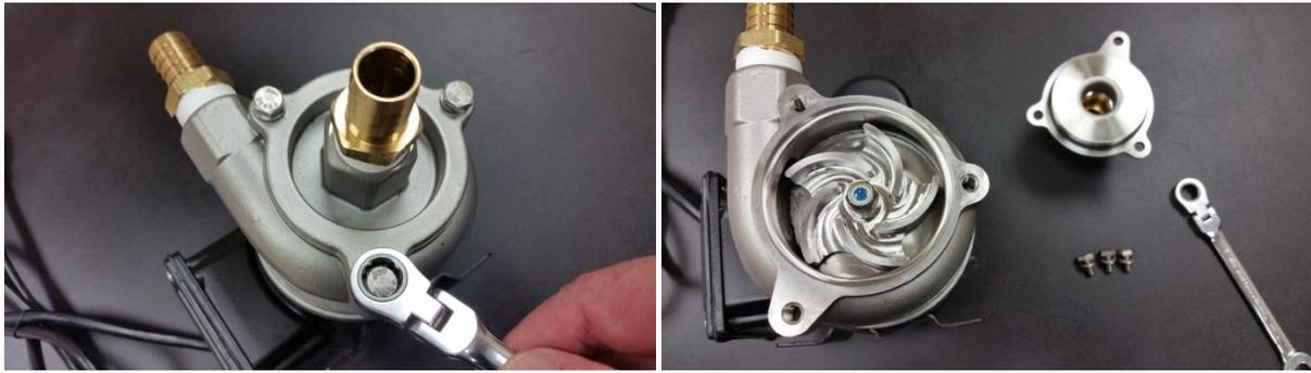
After removing the pump from the machine, remove 3 bolts and lock washers holding pump cover on.
