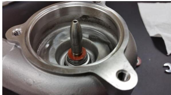
Carefully press the seal down the shaft until seated against the white ceramic portion of the seal. Do not pound or hammer on the installing tool, this could break the ceramic portion.
