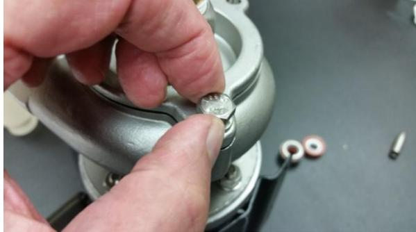
Align the cover, insert the 1/4-20 SS bolts and lock washers, tighten firmly. Remove the plug on the end of the motor cord and attach motor wires to the original wires of the machine control for the drain pump.
