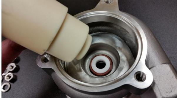
Place the ceramic portion of the seal, boot down into the housing. Use small amount of dish soap.
