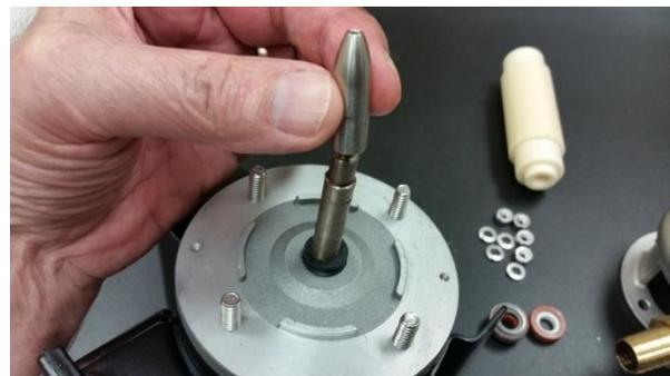
Turn the housing over, check that seal and boot are fully seated in housing, place protective shield over the threads on the motor shaft.
