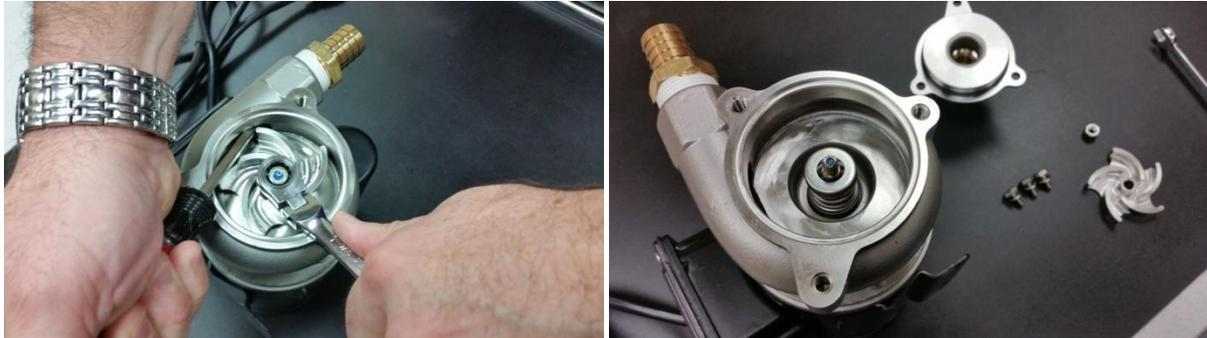
Brace the impeller against a screwdriver to remove the locknut holding the impeller to the shaft.
