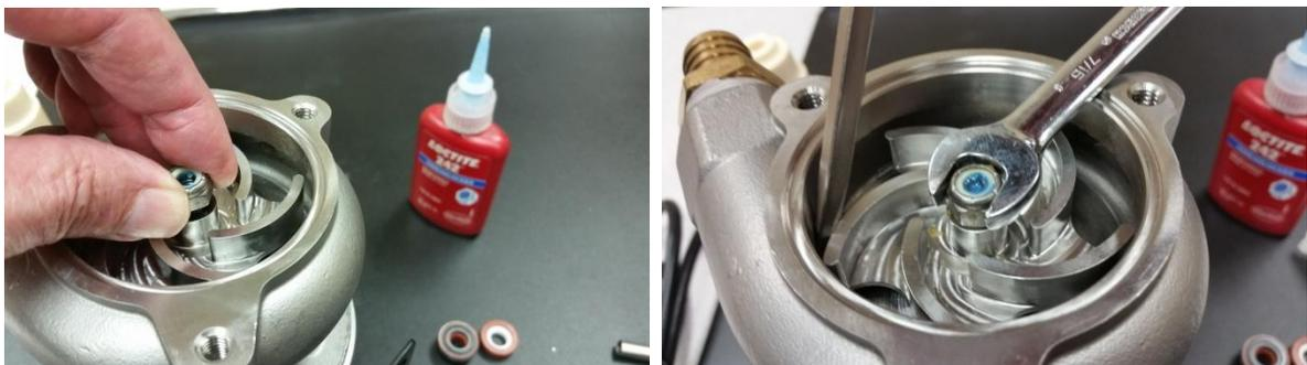
Place one drop of Loctite on shaft threads. Brace impeller with a screwdriver and fasten locknut 098-2507 to hold impeller securely to the motor.
