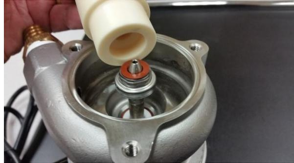
Also lube the protective shield covering the threads, slide the seal on the shaft, use open side of the tool.
