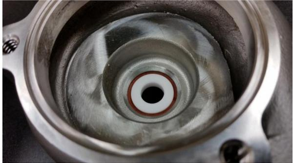
With tool 088-1092 press the ceramic firmly to the bottom of the housing.
