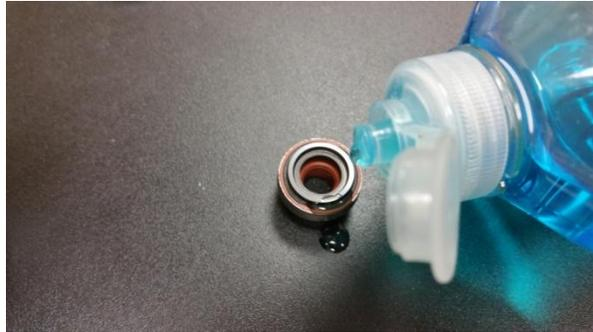
Place lock washers and nuts on the studs and tighten. Place small amount of soap on black portion of seal.
