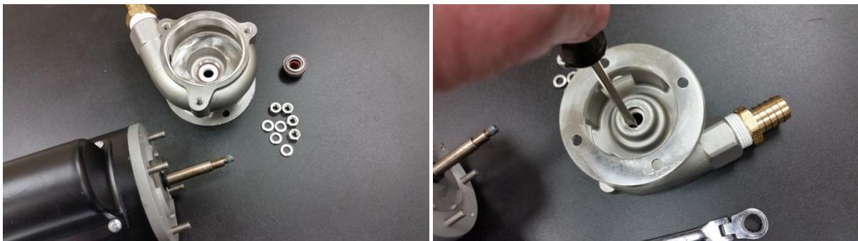
Lift the pump housing off the motor; from the back of the housing push the ceramic portion of the seal out.
