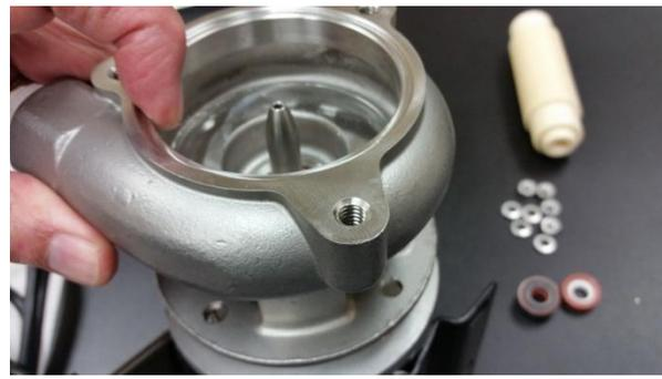
Carefully place the housing on the motor, align the housing correctly and slide it over the 4 attachment studs.
