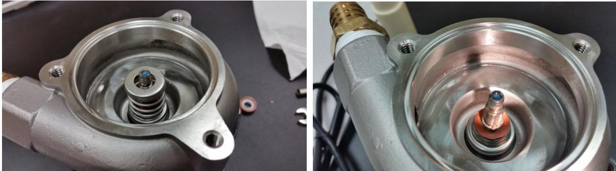
Look closely at the shaft to see the side machined with a flat; this must be aligned with impeller.
