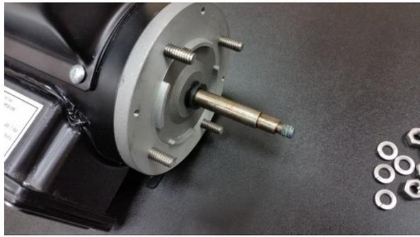
With two seal parts removed and housing off of the motor, the new motor can be put into the assembly.
