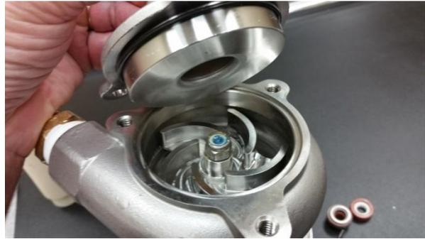
Place O-ring gasket 089-6311 on the pump cover and place into the pump housing
