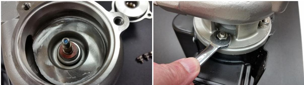
Take the spring and cap out, remove the 4 nuts and washers holding the housing to the motor.
