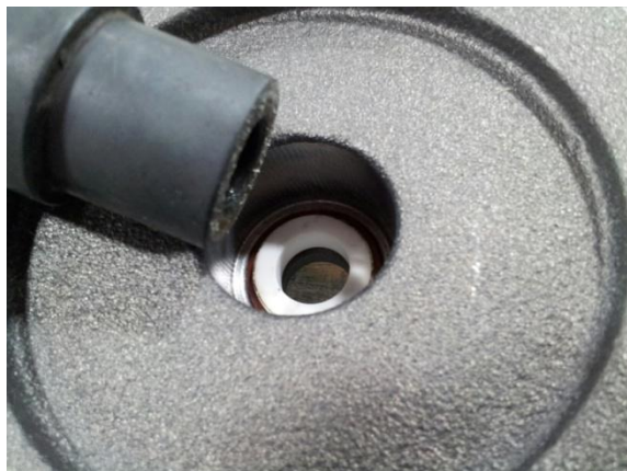
Installing tool #099-6007 to press to bottom of bore
