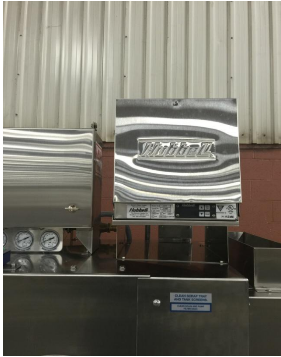
Front view of Right to Left conveyor, booster always on soil side
