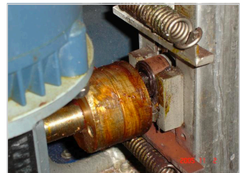
Cam bearing and springs of conveyor
