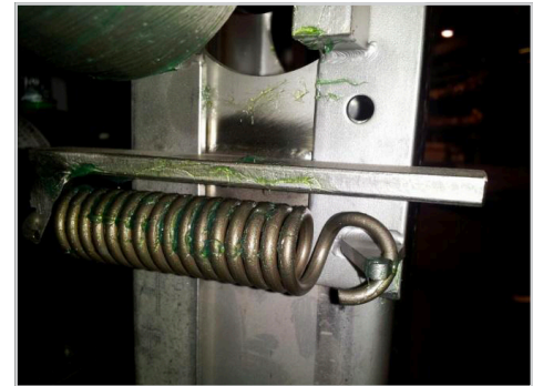
Conveyor arm slip-clutch spring
