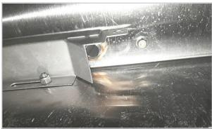
By moving the deflector so it covers half the pipe exit tube, water would be deflected towards the rinse tank.
