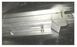
Please note in picture #1 looking up, the adjustment studs are shown at the far right of the slots (meaning the diverter duct is moved to the far left for this machine--a R-L conveyor) and the water pipe exit is fully open to drop into the wash tank. Adjusted as shown means the rinse tank would receive no water and the machine would continually fill, not shutting off.
