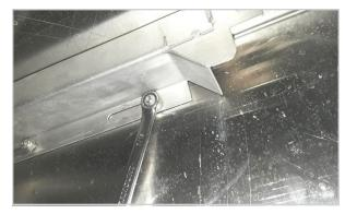
How to adjust the diverter duct, loosen both nuts holding the plate to slide left or right
