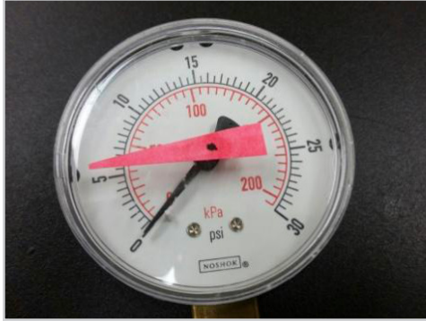
Lower wash arm pressure approx 5-6 psi
