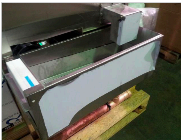
Scrap box is mounted on the right of machine
