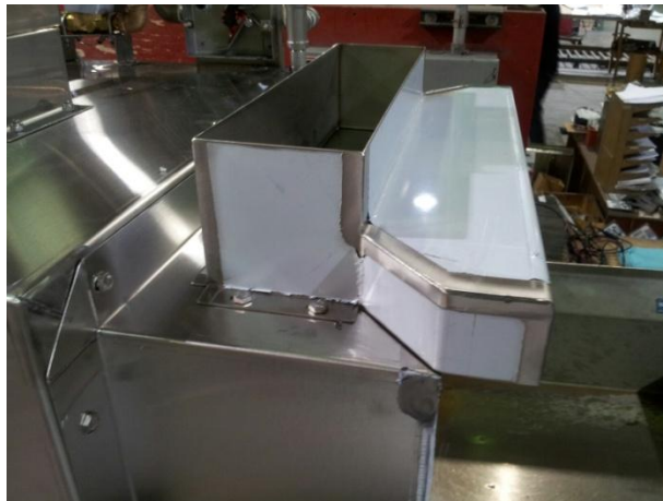
Standard 4" tall (285-6116) vent attachment. Opening is 4x16" and top is 58.25" above finished floor.
