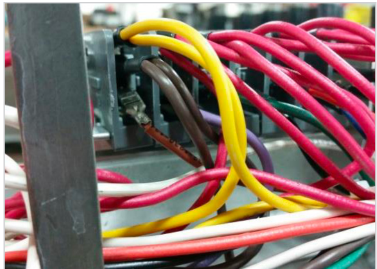
Wire connections made to the 7th switch on cam timer
