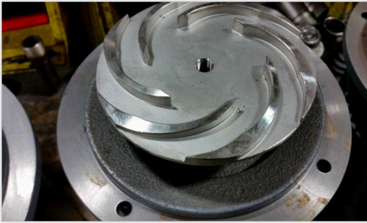
Open impeller (082-6312) 6 vanes modified, 5.0" dia., screws on – right hand thread Pump cover–stud mounted (082-6307), Rear housing (082-6301), Shaft Seal (092-2001), O-ring gasket (089-6309) Used on: AF-ES & AFC-ES 1.5hp pump w/motor 091-1001 and 5AGES 1.0hp pump w/motor 091-1024
