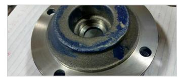
Now with the aux shaft attached, place the pump housing (282-6307) to the motor.
