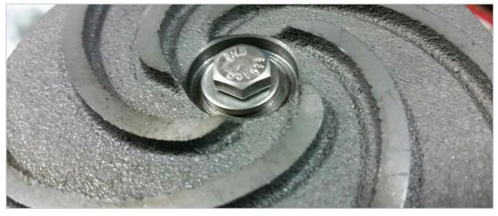
Then twist the impeller to the right as looking at it from this picture, when it seats hand tight, place the secure bolt and washer (098-1443, 098-2413) in the end of the shaft and tighten.
