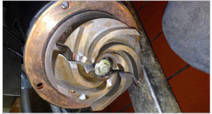
Results of key shifting in the shaft and motor
