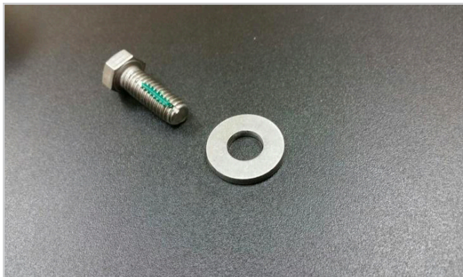
This bolt should only be used once, and never reused
