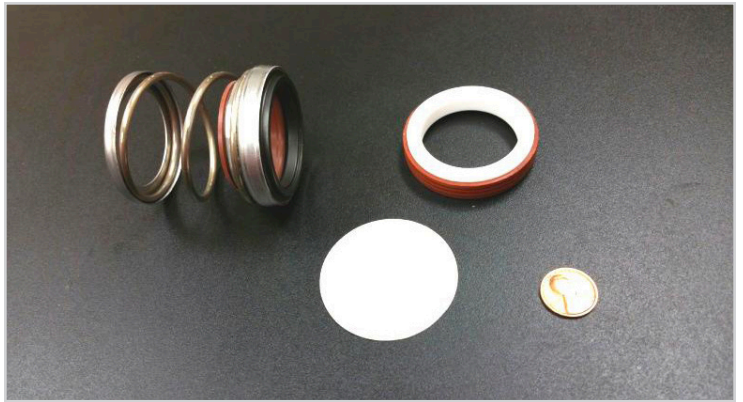
Seal spring, graphite half, ceramic half and rubber boot
