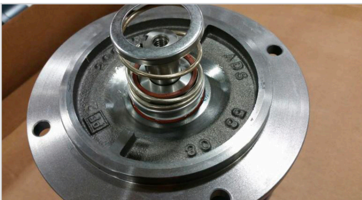
Using dish soap again, press graphite till it seats on ceramic
