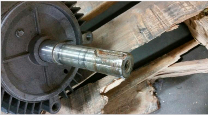
Showing key way damaged
