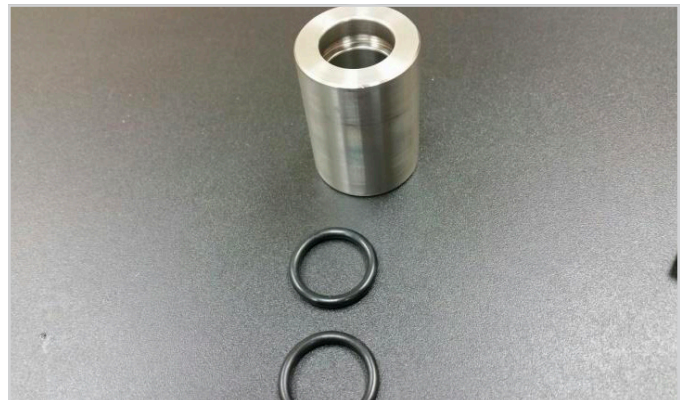
Motor shaft sleeve w/inner o-rings
