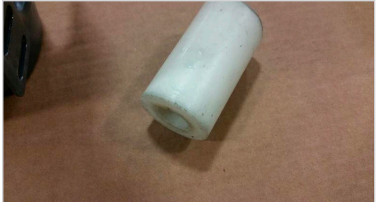
Use 1.5" OD plastic tube to press seal till firmly seated
