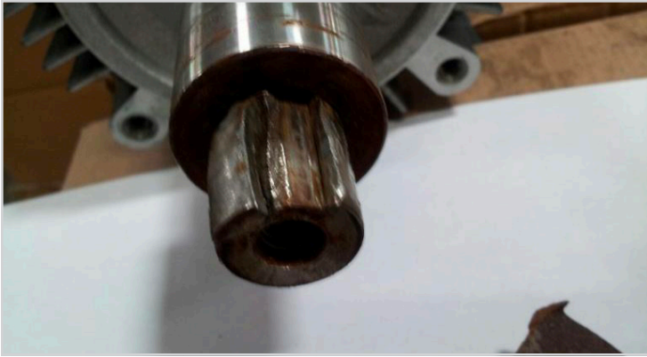
Motor with damaged key way
