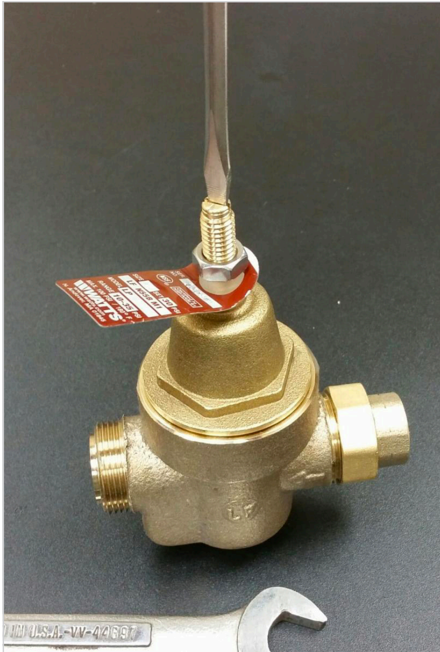
After loosening the lock nut, turn the center rod out (left) to reduce pressure.
