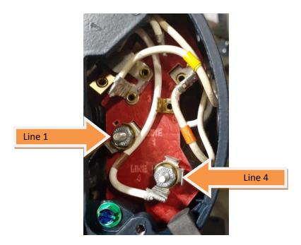
Incoming power Line 1 is attached to line1 spade connection on the motor terminal connection plate. Incoming power Line 2 is attached to line4 spade connection on the motor terminal connection plate.
