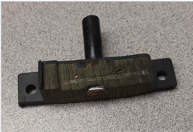
A typical reed WITH printed circuit board
