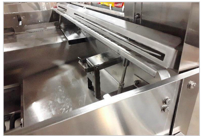
A broken or leaning front tray track will push the magnet pendulums out into the tank, this will cause the motors to keep running after a rack exits the machine. See above
