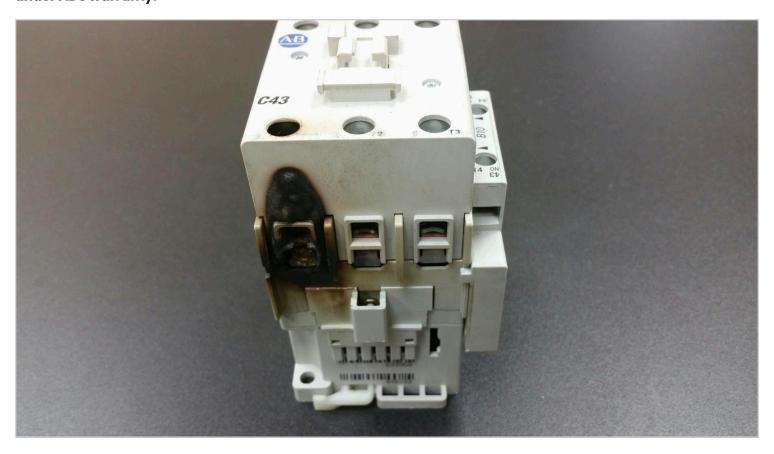
Burned wires on a high amperage circuit, occurs when that circuit experiences interference with the transfer of electrons across conductors, connections, points, or terminals. When it is difficult for electricity to pass over or through a material, that restricted flow will heat up the surrounding material. This flow restriction is called resistance; you experience this when you slide across a hard wood floor on your knees. Resistance causes heat. This is an elemental
