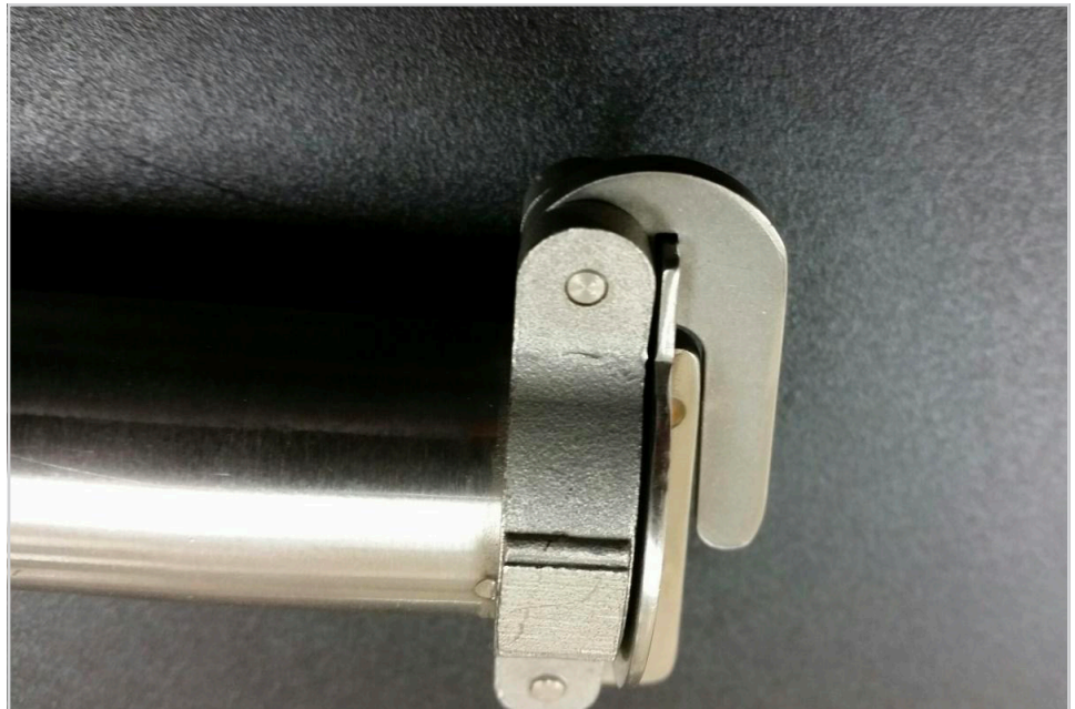
Showing a tight snap-action captive endcap in the closed position. When the endcap is closed properly, it is normal for some water to spray out from around the cap; this will act as the last spray jet on the arm.
