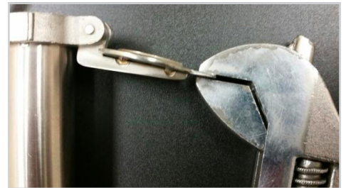
The tab is now straight with the coin edge
