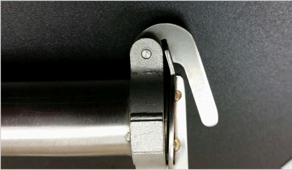
This picture shows a loose endcap that won't stay closed because the tab is bent in toward the tube.
