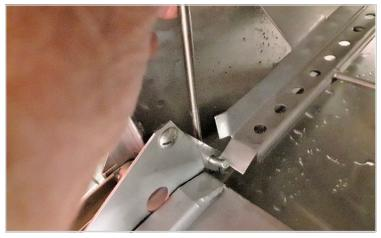
If the spring should break or bolts loosen, the tool will be needed to pull the smaller link up to align with the bolt hole on the rail of the door. This is done by hooking the open end of the tool through the open hole on the smaller link from behind the tray track (see photo above).
