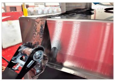
Then using the ratchet, draw the link upward until the hole of the link and the hole on the door rail align. When tightening the bolt, make sure that 1 to 2 threads are showing through the lock nut.
