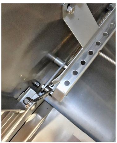
Then using the ratchet, draw the link upward until the hole of the link and the hole on the door rail align. When tightening the bolt, make sure that 1 to 2 threads are showing through the lock nut.
