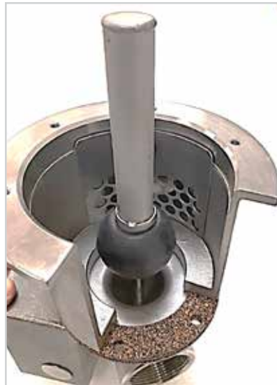
New 2024 arrangement for the inside sump drain ball operator, no wingnut attachment.
