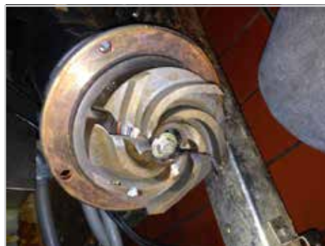
Damaged impeller from excessive start/stop
