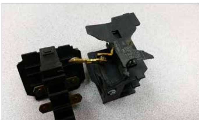
Showing inside of the contactor where contact points burned together (welded). This was caused by loose screw terminal.
