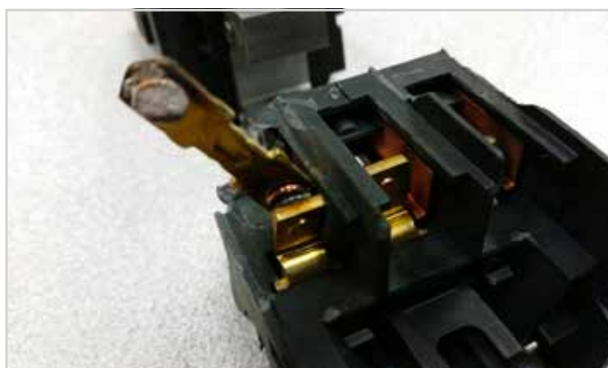
Showing inside of the contactor where contact points burned together (welded). This was caused by loose screw terminal.
