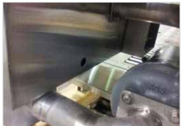
Showing 7/8" detergent probe hole behind pump motor
