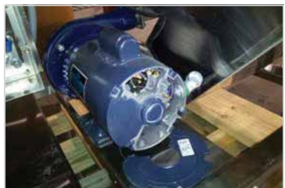
66 power scrapper motor, 1.5 HP, 208v, single-phase
