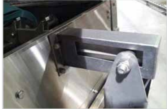
Rocker arm attached to conveyor bar, drip chute
