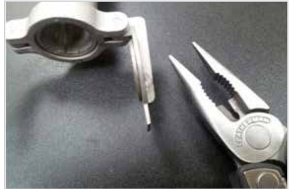
Straighten tab in line with the coin edge to tighten latch
