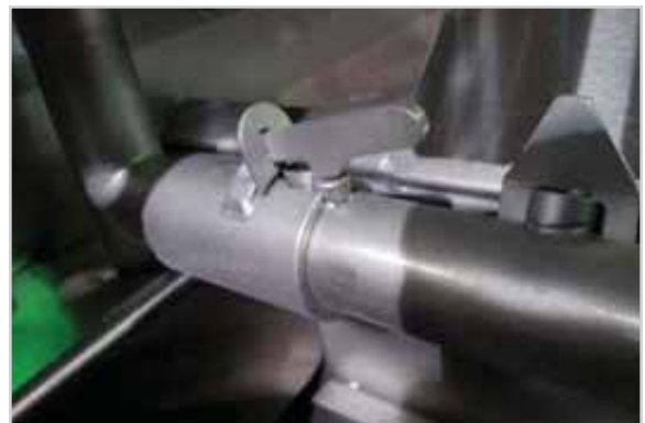
Rinse arm index notch, latch will drop as arm is pushed in
