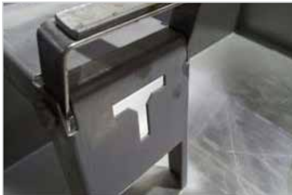
Showing wash arm T index for lower arm
