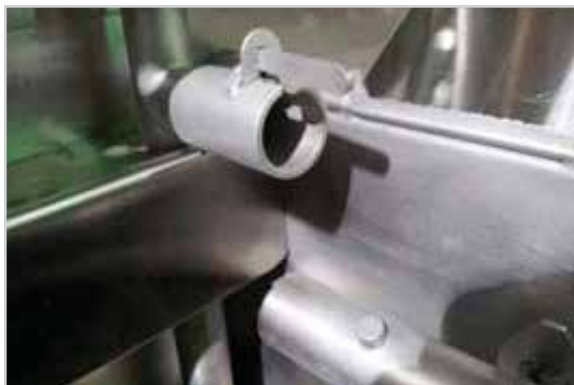
Showing pumped rinse manifold locking tab
