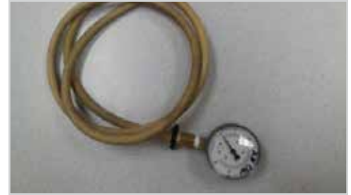
Spray arm pressure tester #088-1048
