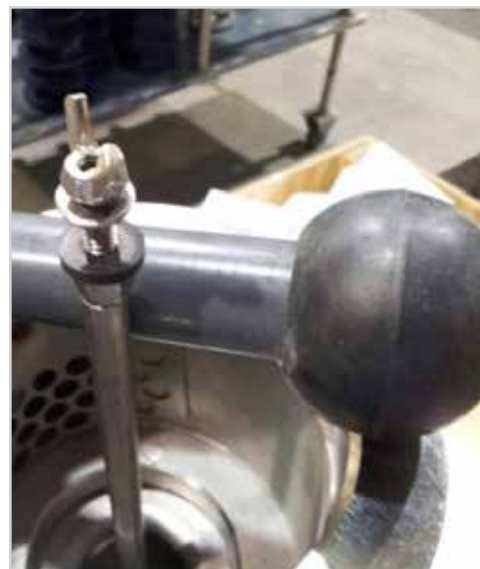
ET (gravity) drain ball, note rubber washer on push rod
