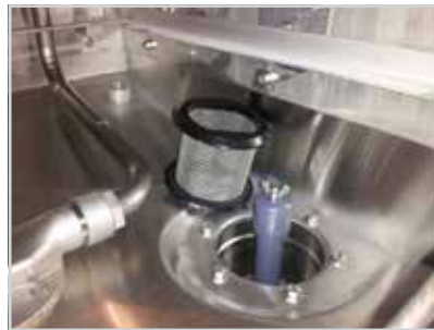
Drain ball assembly and pump filter
