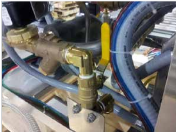
Showing 1/2" female pipe inlet, ball valve, y-line filter, H2O solenoid
