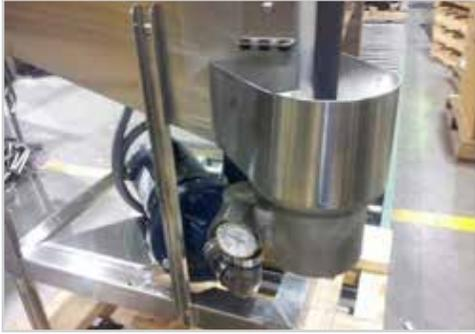
Showing AF-ES sump, drain ball, thermometer
