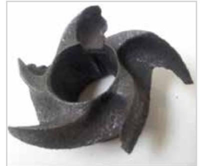
Impeller damaged from high acid solution
