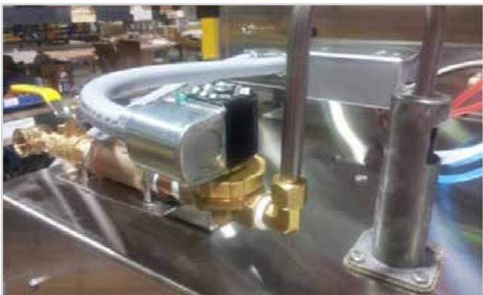
Showing 1/2" female pipe inlet, ball valve, y-line filter, water solenoid, ASSE approved air gap (backflow preventer)
