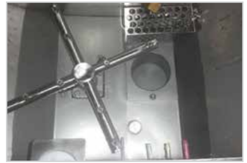
Wash tank with spray arm, float, secondary scrap screen
