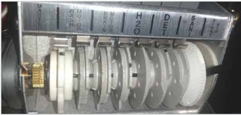
ASQ II cam timer, fixed cams are MASTER, WASH MOTOR and DRAIN MOTOR
