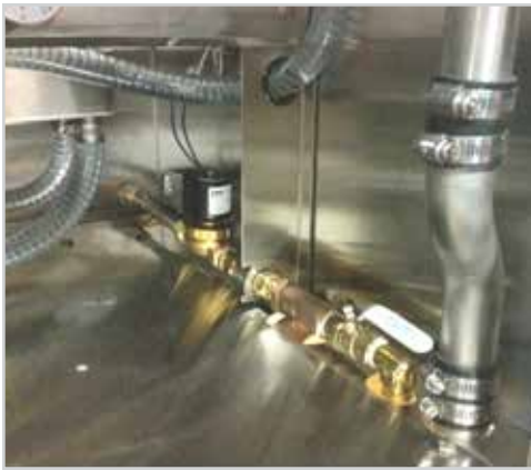
Showing 1/2" H 2 O solenoid, also stainless 1.5" drain tube
