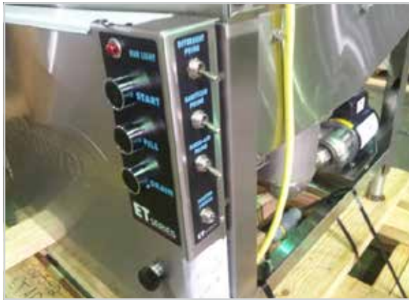
Showing controls on lower access door & drain pump
