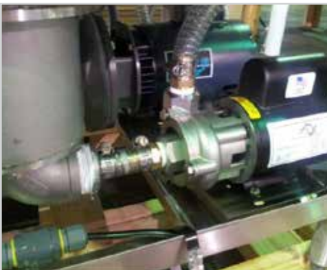
Showing stainless drain pump with 3/4" discharge tube
