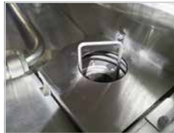
Drain ball assembly and pump filter
