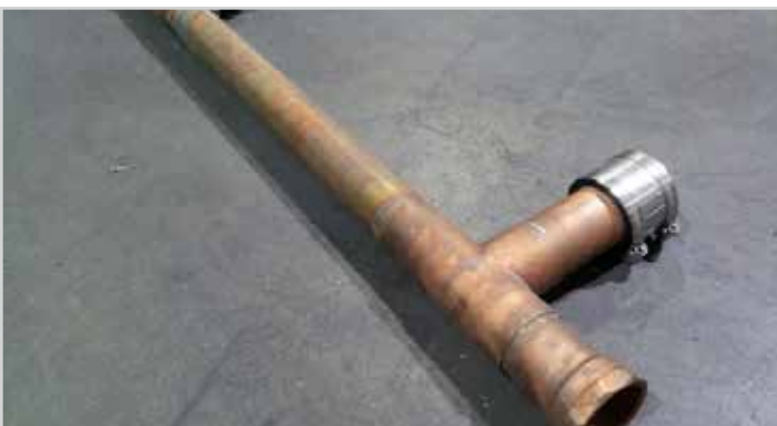
HT-25 drain manifold with "no-hub" connectors
