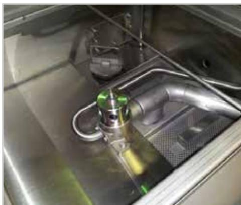
Showing spray arm base & transfer tube
