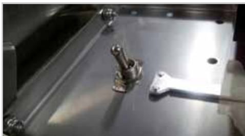
De-lime switch in HT-25 control box
