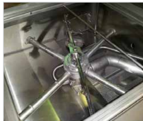
Final rinse arm twisted into transfer tube
