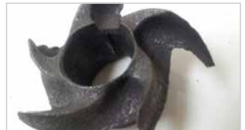
Impeller damaged from high acid solution
