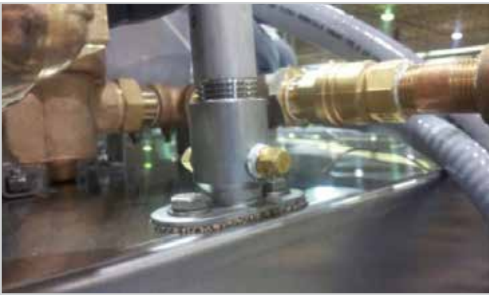
Mixing chamber with two 1/8" pipe threaded port
