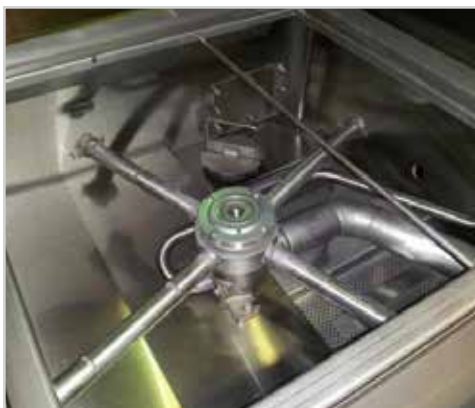
Wash arm w/bearing installed on base
