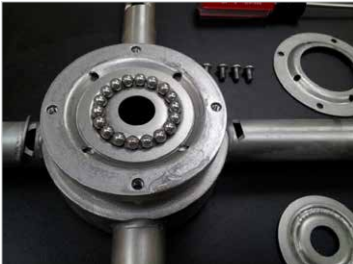
Top race removed, ball bearings for replacement
