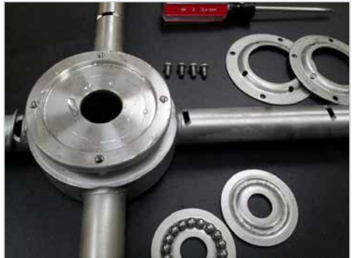
Races are interchangeable, capture shells are also
