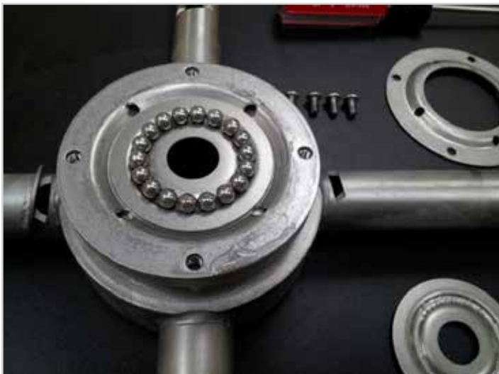
Top race removed, ball bearings for replacement
