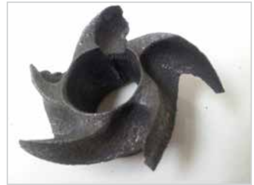
Impeller damaged from high acid solution
