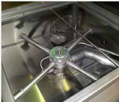
Wash arm w/bearing installed on base
