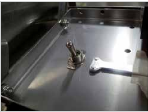
De-lime switch in HT-25 control box
