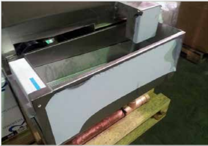
Scrap box and 2" drain manifold attached to pallet for shipping
