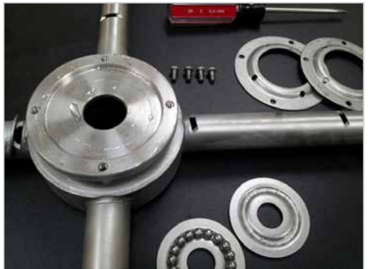
Races are interchangeable, capture shells are also
