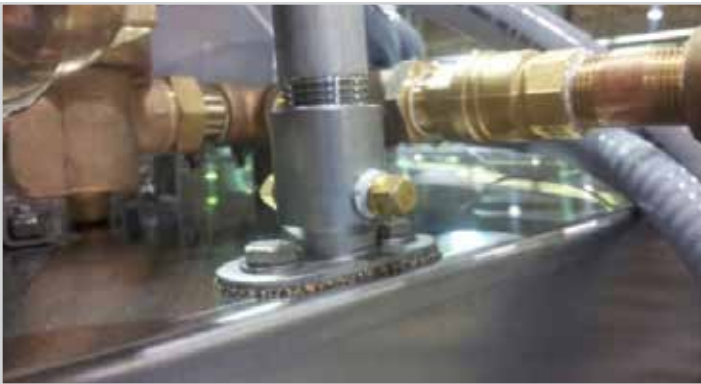
Mixing chamber with two 1/8" pipe threaded port
