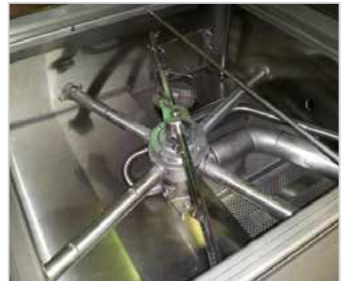
Final rinse arm twisted into transfer tube
