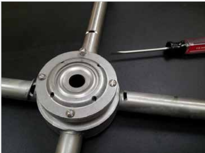
Remove 4 screws and lift top shell
