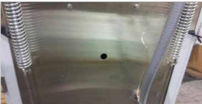
Showing back of tank, 7/8" detergent bulkhead fitting hole
