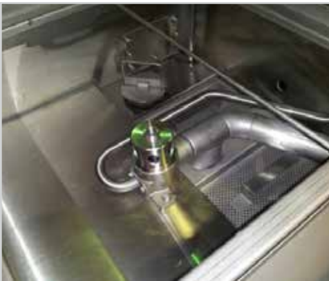
Showing spray arm base & transfer tube
