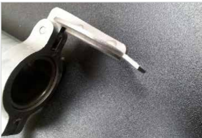
Tab on endcap bent inward, causing loose fit
