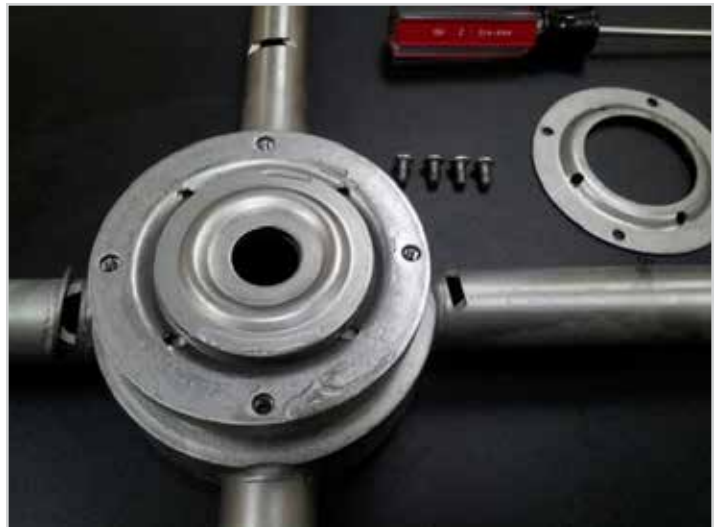
Remove top shell, exposing top bearing race
