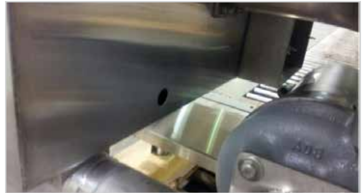
Showing 7/8" detergent probe hole behind pump motor
