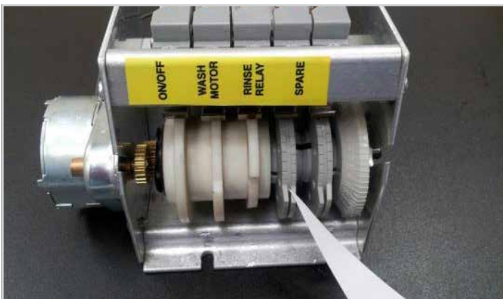
Showing HT-25 cam timer, arrow points to deter cam
