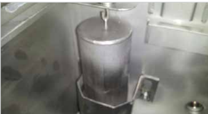
Wash tank float and tank overflow
