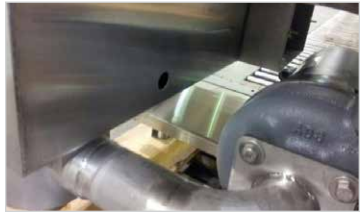
Showing 7/8" detergent probe hole behind pump motor
