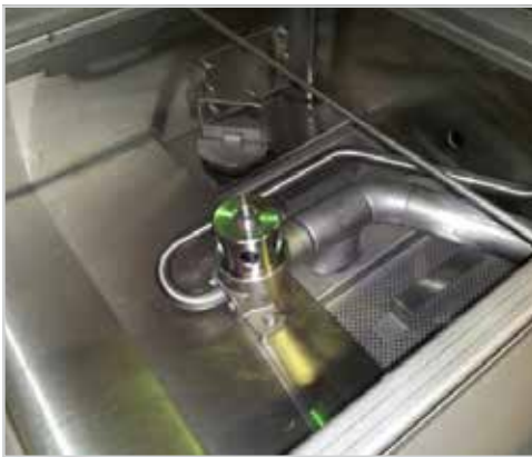
Showing spray arm base & transfer tube
