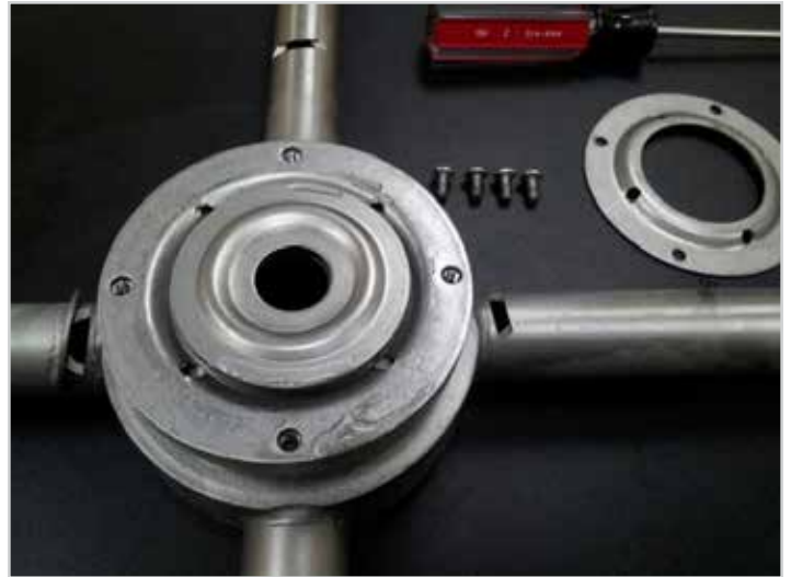
Remove top shell, exposing top bearing race
