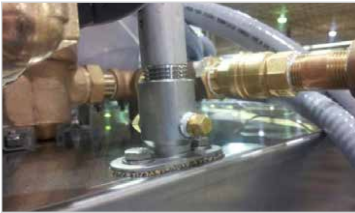
Mixing chamber with two 1/8" pipe threaded port
