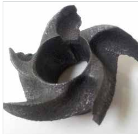
Impeller damaged from high acid solution
