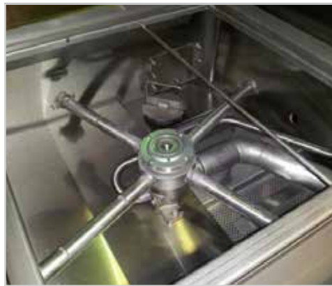
Wash arm w/bearing installed on base
