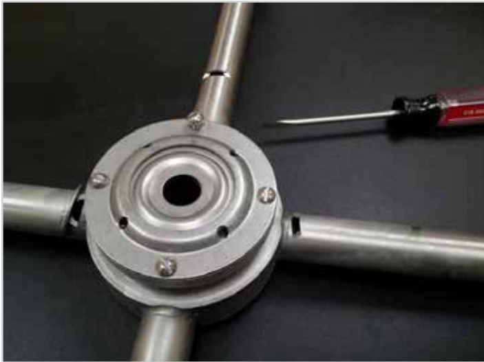
Remove 4 screws and lift top shell
