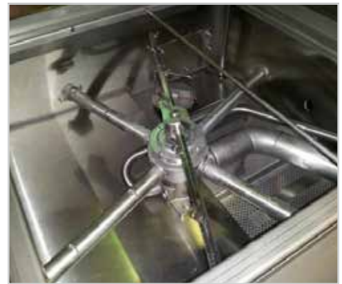
Final rinse arm twisted into transfer tube
