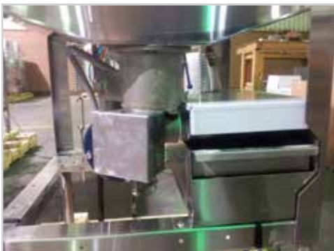
Showing L-3DW-S internal sump and scrap box
