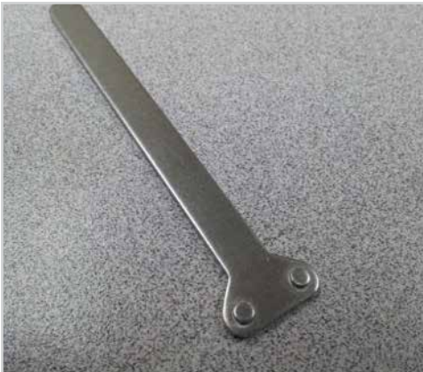
Cam timer adjustment tool
