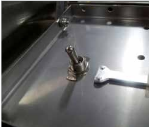
De-lime switch in control box
