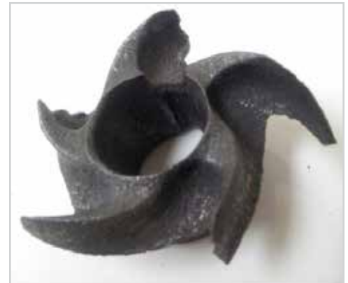
Impeller damaged from high acid solution
