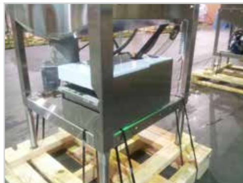
L-3DW-S scrap box in-frame mounting
