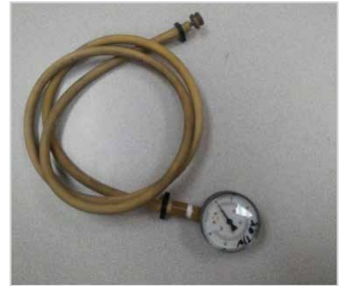
Spray arm pressure tester #088-1048
