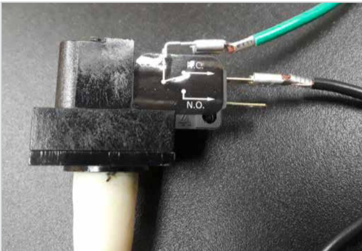
Wire connection to the vacuum switch
