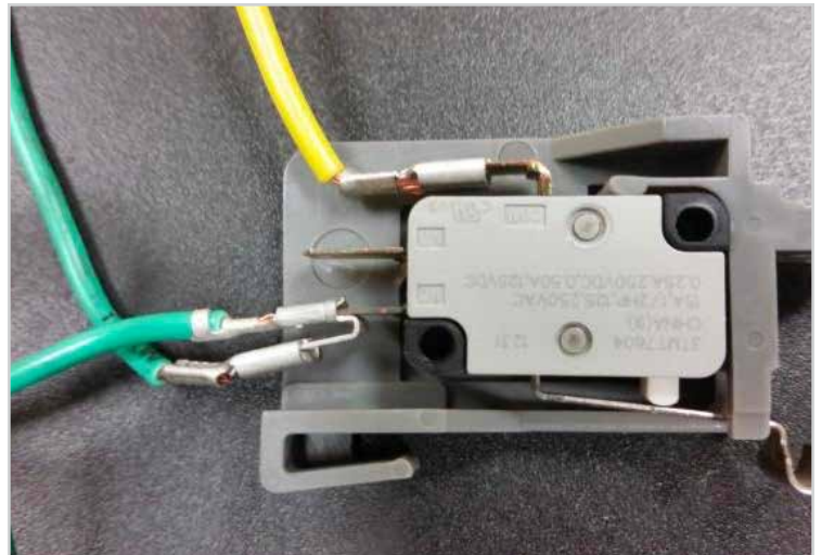
Wire connections to the cam timer sanitizer
