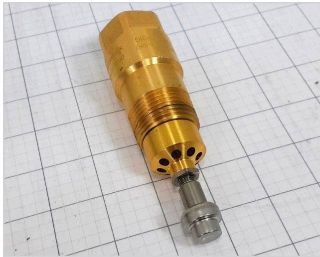
ADS P/N 292-5008 Tempering Valve (Open 130F, Close 120F, max temp 240F)
