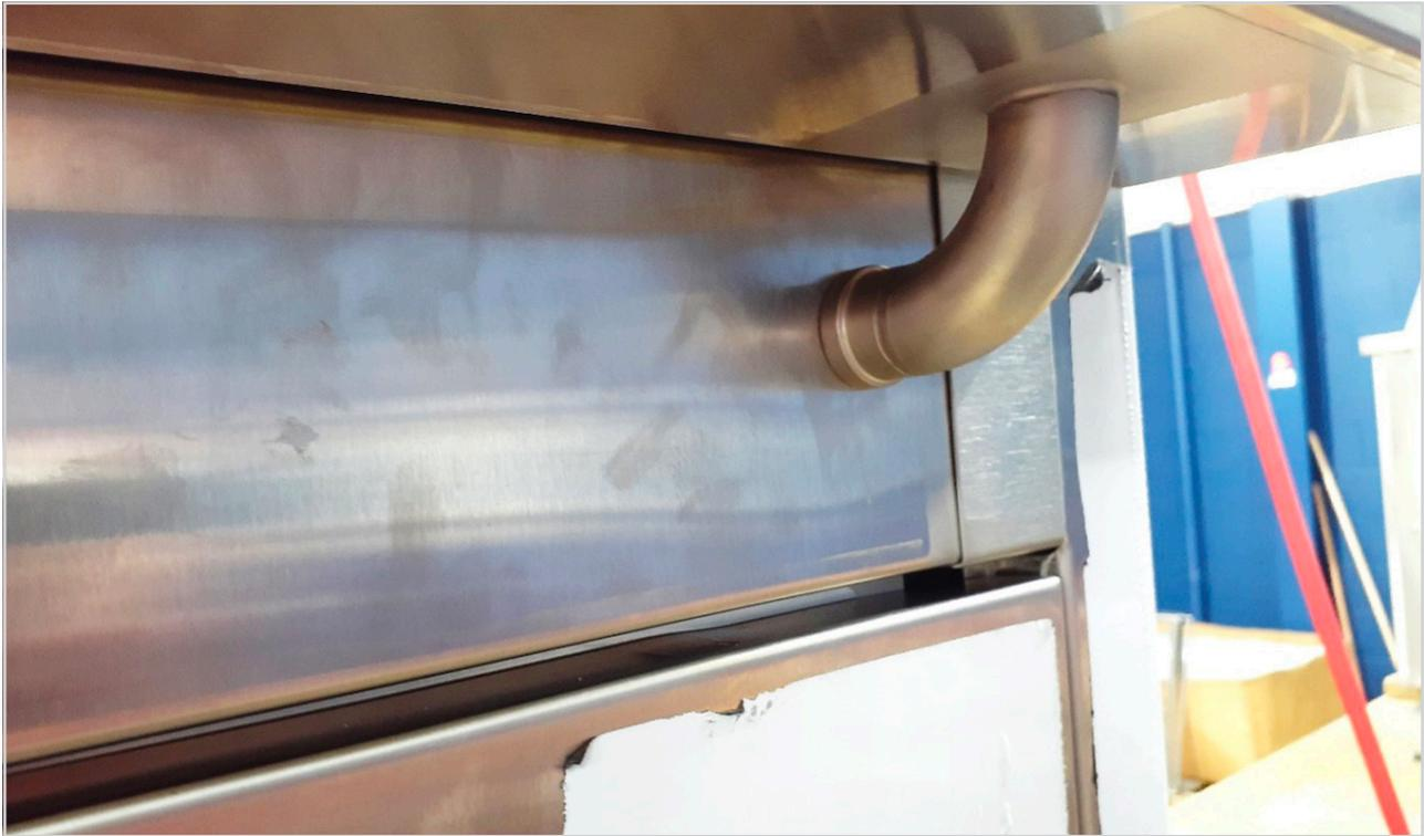
To install, place the dump weldment on the front lip of the ASQII, press down while rotating the elbow's threaded end into the hole in the front of the tank. This holds the weldment in place. To remove, take the brass nut and washers off from inside the tank and pull the elbow out of the hole and lift the weldment off the lip of the tank.
