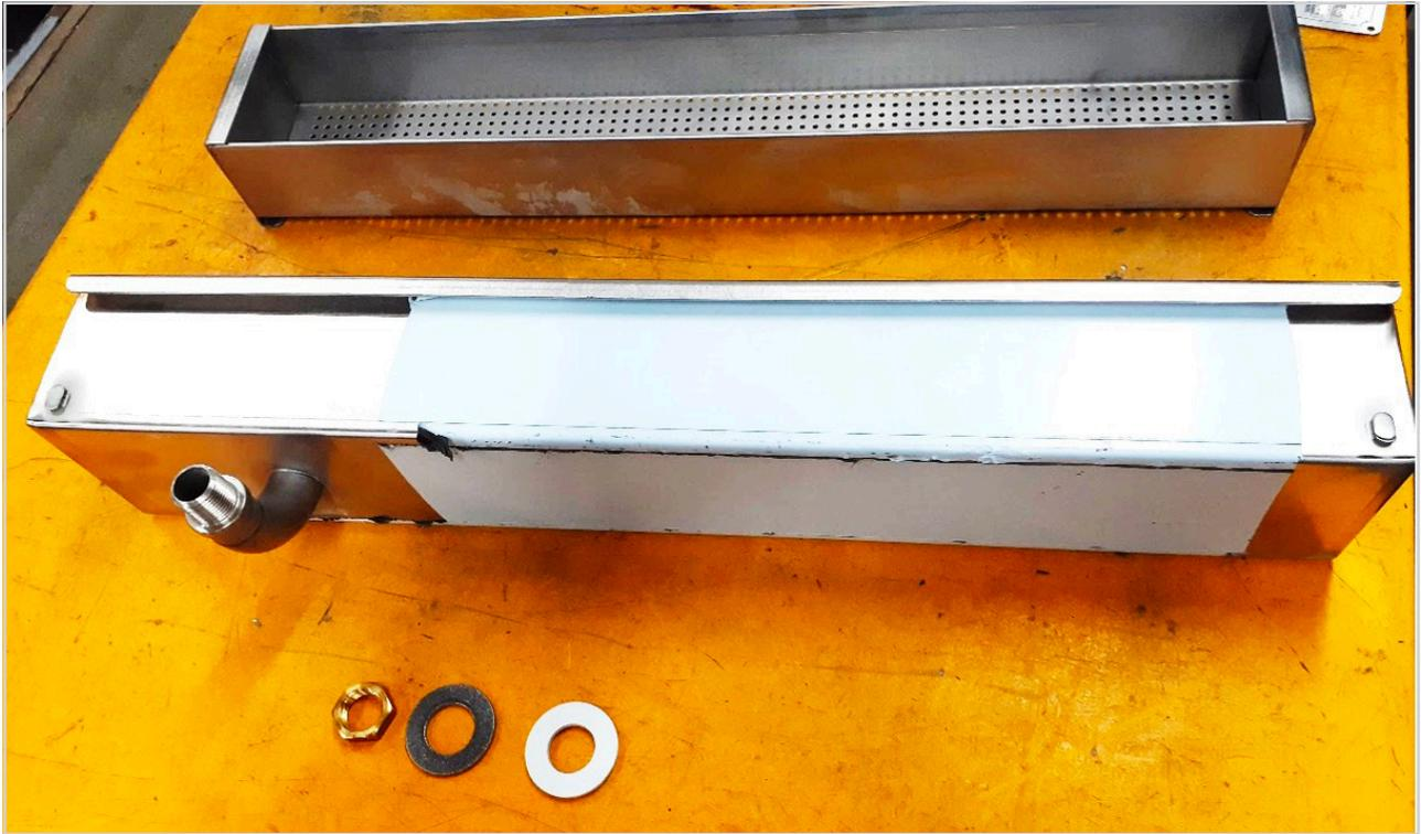
Showing from top to bottom, Dump Tray, Dump Weldment, Brass nut, Stainless Washer, and Rubber Washer.
