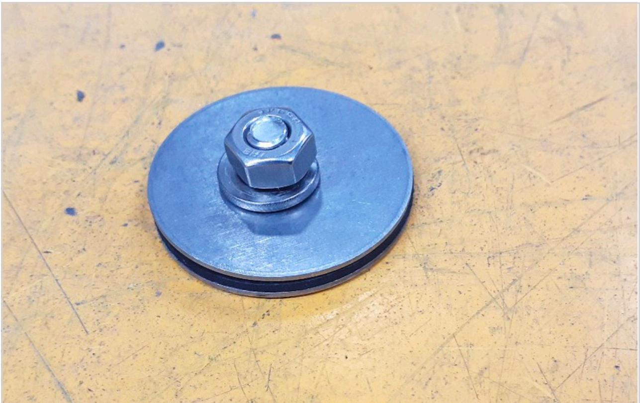
With the Dump Weldment removed, place the probe plug in the open hole and tighten in place as shown below to finish the removal. To install a new Dump Weldment and Tray, follow these instructions in reverse order.
