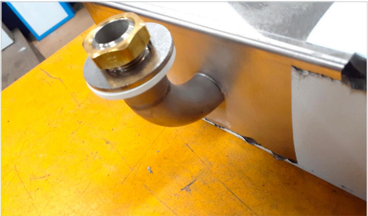
Showing the order in which the rubber washer, stainless washer and brass nut are inside the tank.
