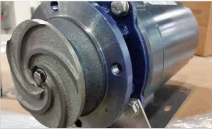
Open impeller (282-6308) 5 vane, 4.0" dia., low profile, screws on – right hand thread w/secure bolt (098-1443) washer (098-2413) Pump cover (282-6306), Rear housing (282-6307), Shaft Seal (292-2002), Fiber gasket (289-6609) Used on: ADC-44/66 for 1/3hp rinse pump w/motor 291-1003
