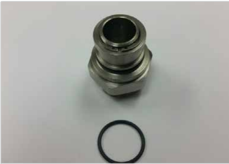
Spray Arm Bearing #081-6217 (cleanable), takes a 1.25" wrench, right-hand thread, with "O" ring #089-6310 (.019)
